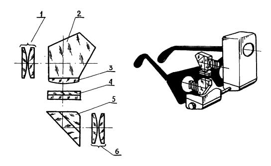
FIGURE 1. Optical scheme of safety goggles: 1-objective lens, 2-pentaprism, 3-collective lens, 4-spatial light modulator, 5-prism, 6-eyepiece.
